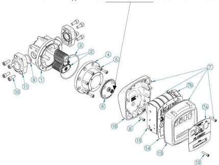
**4.2 Inspection** (*refer Exploded View*) Inspect O-rings for damage, chemical attack, deformity or any form. Remove, inspect & clean the rotors, check that the primary rotor gear pinion for any damage. Check the measuring chamber for damage or scoring & redress if necessary, the rotor shafts should NOT be loose or able to be rotated.
