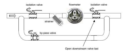
After flushing or following long periods of shutdown the meter must be purged of air/vapour. This can be achieved by allowing the liquid to flow through the meter at a slow rate until all air/vapour is displaced. Never run the meter above its maximum flow or exceed 100kpa (1 bar, 15psi) pressure drop across the meter. Now the meter is ready for its operation to be confirmed by ensuring correct indication on the mechanical display. Refer if necessary to fault finding section of this manual.
