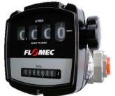
Liquid can flow into the meter from either a horizontal or vertical direction. For vertical flow installations the most common orientation is for the liquid to rise through the meter (i.e. travel from bottom to top) to assist in air or entrained gas elimination. Be sure to observe flow direction Arrow marking.
